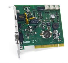
The module supports several transmission formats with automatic recognition and autonegotiation of the communication protocol. The amount of data received by the card is unlimited and their correctness is tested as they come. The card has a FIFO buffer for 250 last received events.
